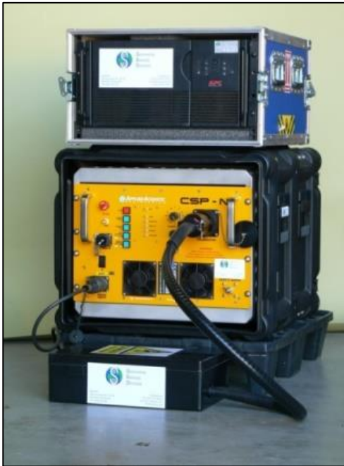
Applied Acoustics CSP-N series HV power supply with UPS unit (on top) and connected HV Junction Box (in front).
