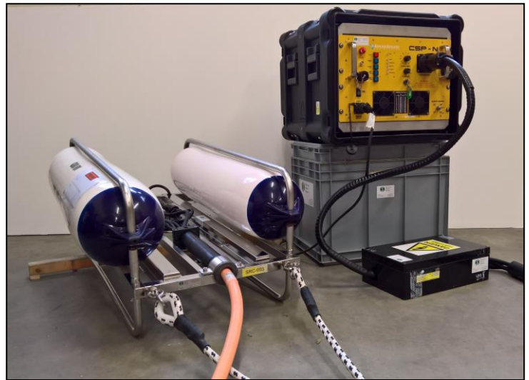
Complete GSO 180 sparker system with HV tow cable, HV junction box and CSP-N Power Supply.
